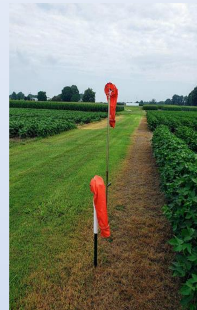
Tall and Short Passive Windssock Spore Samplers
