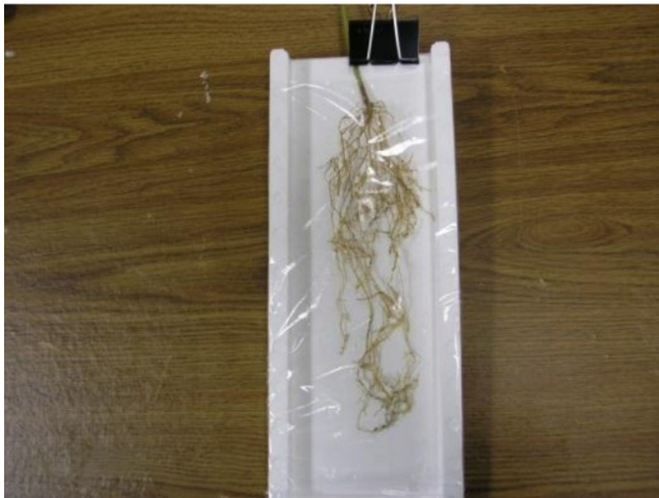
Figure 10. Washed Roots Were Then Prepared for X-ray Imaging
